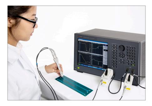
The E5063A PCB Analyzer consists of a E5063A ENA Vector Network Analyzer with Option 011 (Time domain analysis/ Test Wizard). The E5063A provides frequency domain measurement capability and Option 011 adds time domain analysis capability, as well as a dedicated graphical user interface for PCB manufacturing test.
